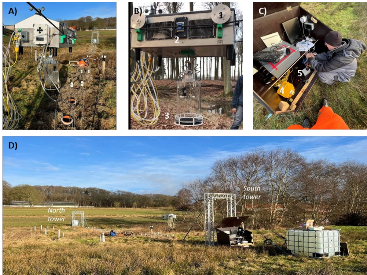
Figure S2: A) The SkyLine2D trolley and chamber at Vejrumbro site looking from south towards the north tower. Note the orange collars on the ground arranged in a straight line. B) Close-up of the chamber: wheels move the trolley back and forth on the ropes (1), magnet sensors (2) and rubber gasket on the bottom of the chamber (3). C) The GHG analyzer “hut” with the Picarro G2508 gas analyzer (4) and the main pump (5). D) The SkyLine2D system with the north and south towers and the GHG analyzer shelter. Towers were at both ends attached with ropes to water-filled 1000 L pallet tanks. One tank shown at the right of the picture.
