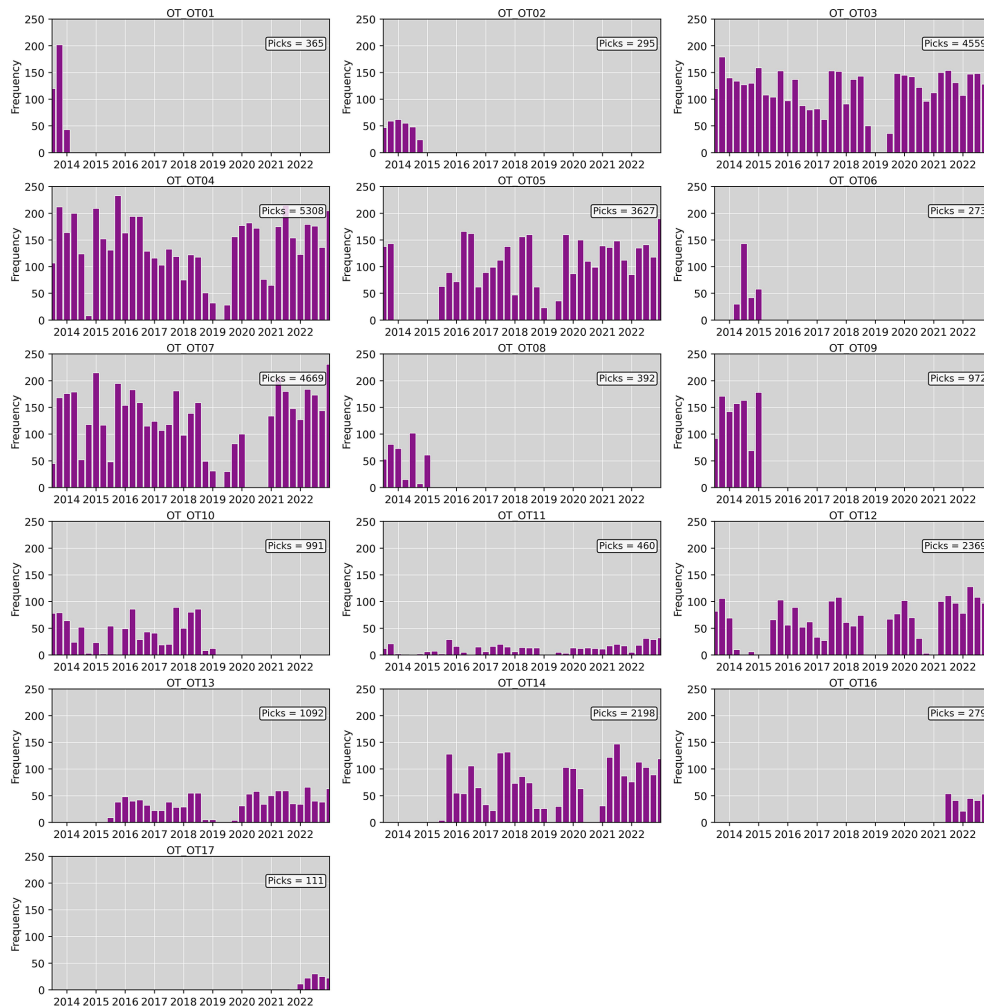
Figure A2. Histograms of number of automatic picking, used for EQ catalogs, for each station of the OT network, from 2013 to 2022 with bins of three months. Superimposed the total number of P and S pickings.
