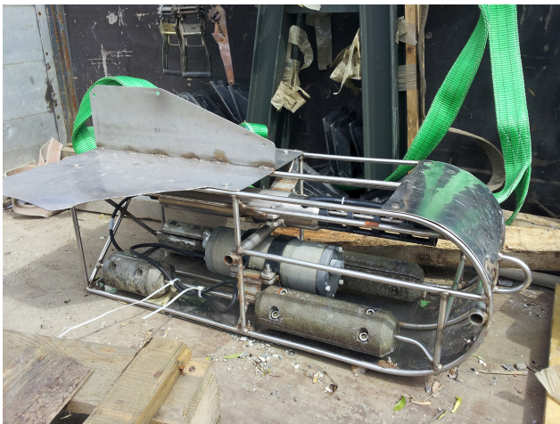
Figure 2. CTD towed probe system used for the collection of data with Sea-Bird SBE49 (2002–2020).
