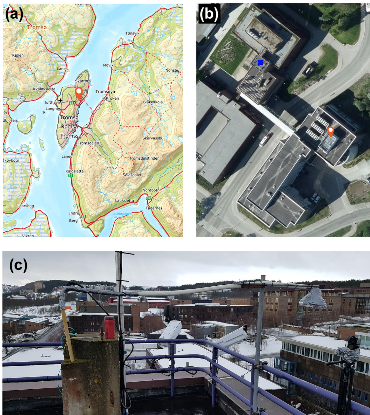
Figure A3. (a) Tromsøya with the location of UiT, and (b) the Natural Science building at the university campus, where the blue square denotes the position of the air inlet and AWS. (c) Ambient air inlet for water vapour isotope measurements on the roof of the University of Tromsø natural sciences building. The maps in (a) and (b) are from https://norgeskart.no/ (last access: 8 April 2026).
