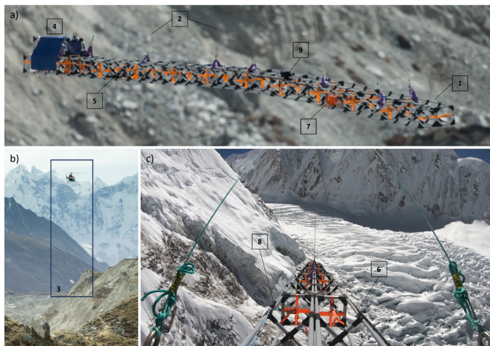
Figure 1. The radar frame consisting of lightweight fibreglass modules strapped together (1), with rope lines (2) to suspend the system under the helicopter (3), a tail (4) to prevent “weathercocking”, a pulse transmitter (5) and corresponding, resistively loaded transmit dipole antenna (6), receiver (7) and receive antenna (8) and GPS (9) (Pritchard, et al., 2020). Panel (c) shows the system approaching the icefall on Khumbu Glacier (Fig. 2), with multiple potential sources of radar clutter notably from the surrounding mountains and crevasse walls. Photo credits: Hamish Pritchard.
