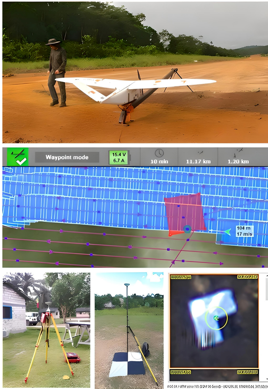
Figure 11. UAV-LS acquisitions at FBRMS-02: Lopé using a fixed-wing system. This UAV employs a conventional take-off and landing (CTOL) procedure, with launch aided by a catapult (top). Once airborne, the UAV is controlled from a laptop connected to the UAV via an antenna (middle). The flight trajectory is corrected to centimetre precision using data collected from a static GNSS receiver placed within 10 km of the UAV operating area (lower left). Additional refinements and corrections are possible via ground control points located across the study area (lower middle), the positions of which are measured using a “rover GNSS receiver (lower right). Image originally published in McNicol et al. (2021).
