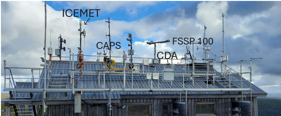
Figure 1. ICEMET, CAPS, CDA, and FSSP-100, installed on the roof at the Sammaltunturi site for PaCE 2022.
