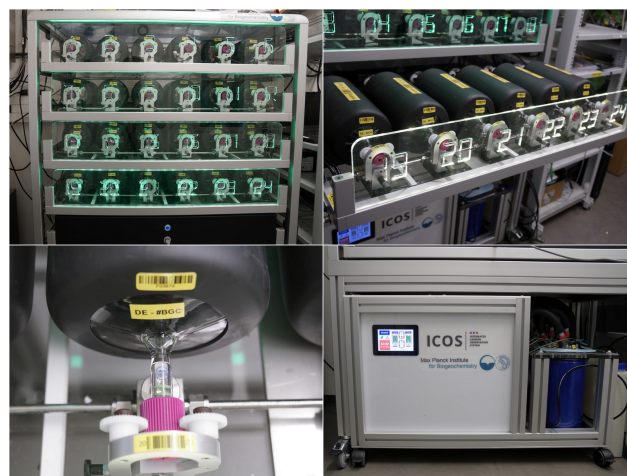
Figure 1. Automated flask sampler installed at the ATTO site. The sampler consists of four trays, and each tray holds six flasks, for a total of 24 flasks available for sampling. A drawer below the last tray contains all the electronic components and the compressor pump. The flasks are of 3 L volume and samples are stored at an overpressure of \sim 0.7 bar. A drying unit (bottom right) takes the air drawn in by the sampler and cools it to a dew point below -38 °C.
