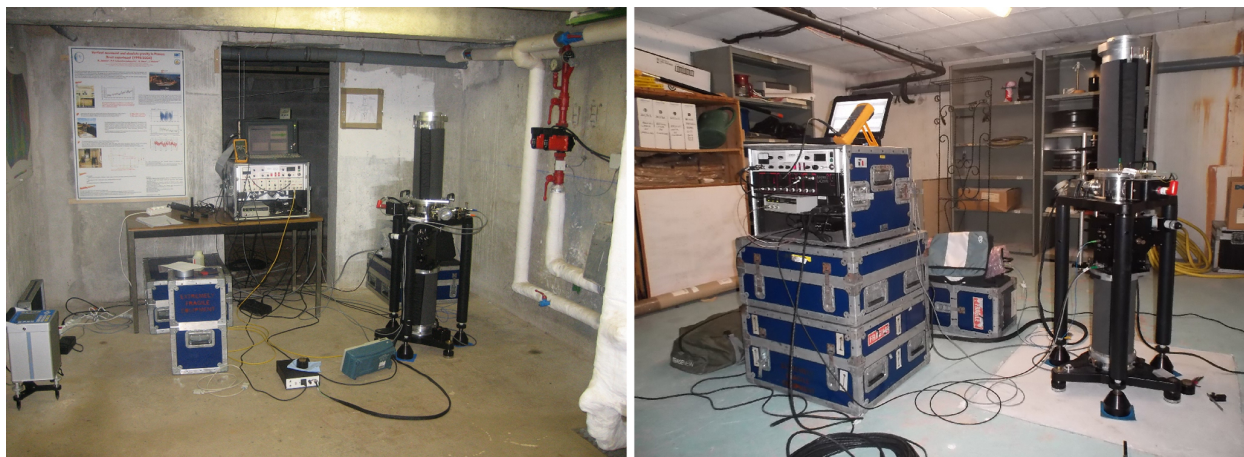
Figure 2. FG5#228 absolute gravimeter observing at Shom in Brest (France) above Ref01 ground floor marker in August 2007 (left) and above Ref02 marker in July 2022 (right).
