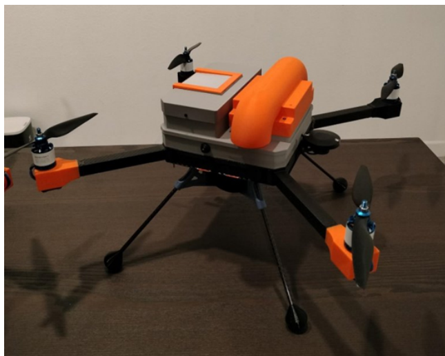
Figure 11. The Oklahoma StormTrooper: an Unmanned Aerial Weather Measurement System (WxUAS) with its remote (left) and in situ (right) payloads. Deployed during 2023–2024 at the GAIL site.
