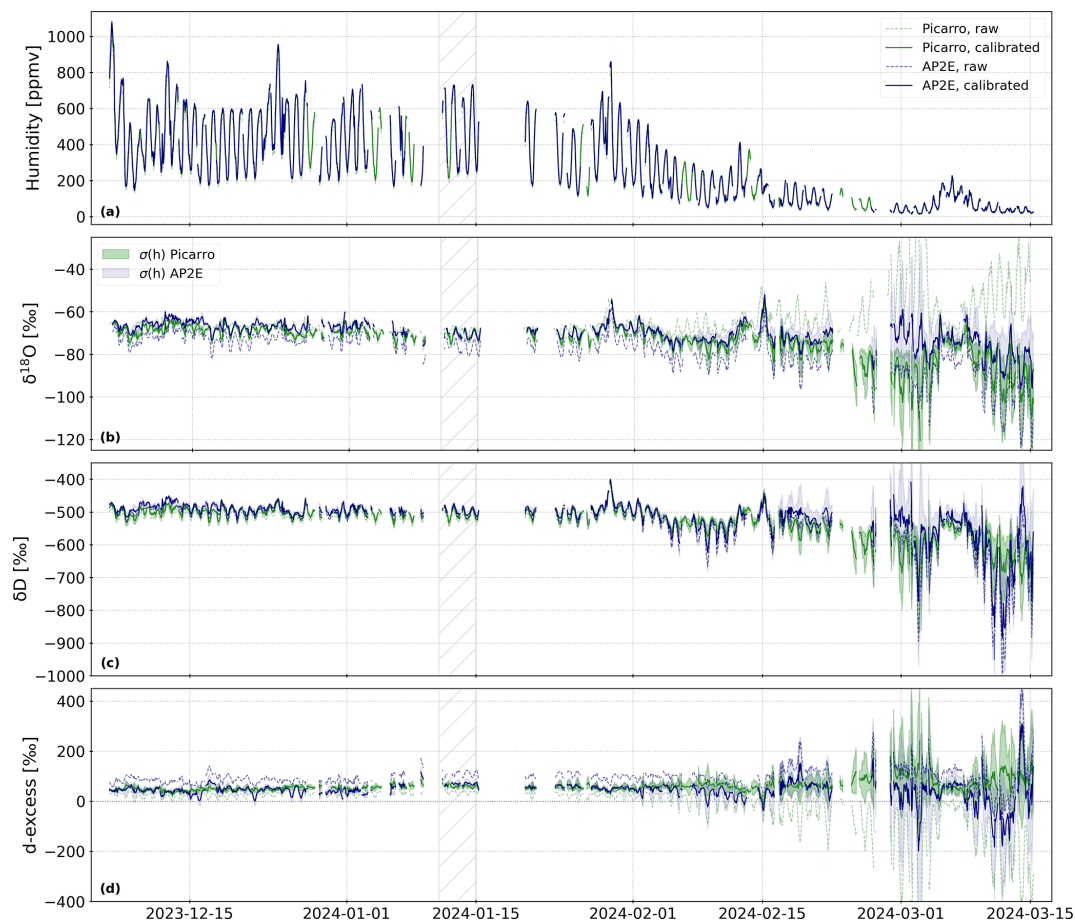
Figure 6. Time series (6 December 2023 to 15 March 2024) of the atmospheric humidity (in ppmv, a ), \delta^{18}\text{O} (in ‰, b ), \delta\text{D} (in ‰, c ) and d-excess (in ‰, d ) measured by the Picarro (green lines) and AP2E (blue lines) analysers. In ( b ), ( c ) and ( d ), the green and blue shaded areas correspond respectively to \sigma(h) (Sect. 2.2.4) of the Picarro and AP2E analysers. In all four panels, the dashed lines correspond to the raw data given by the spectrometers and the plain lines correspond to the corrected and calibrated data (see Sects. 2.2 and 3.1). The grey hatched area marks the period from 11 to 15 January shown in Fig. 7.
