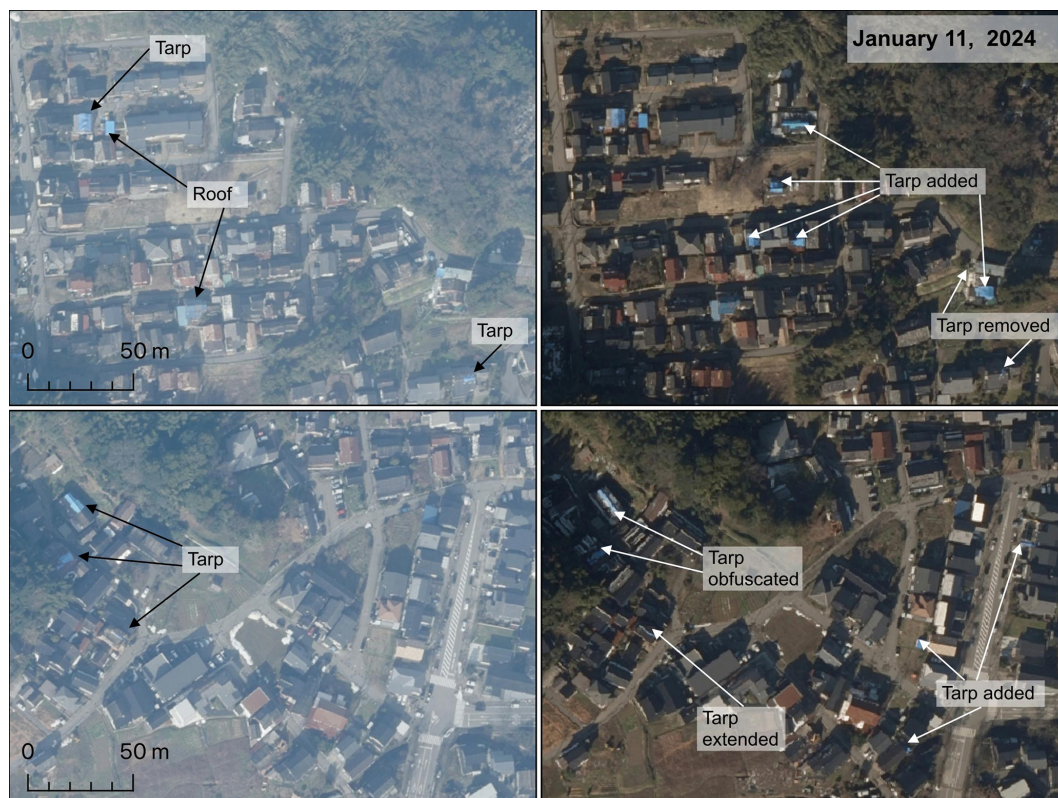
Figure 6. Examples of change in blue tarp coverage in Wajima between aerial imagery capture missions. The figure highlights challenges faced through potential issues with coverage, atmospheric conditions, and source mismatch. Aerial imagery courtesy of GSI (2024).
