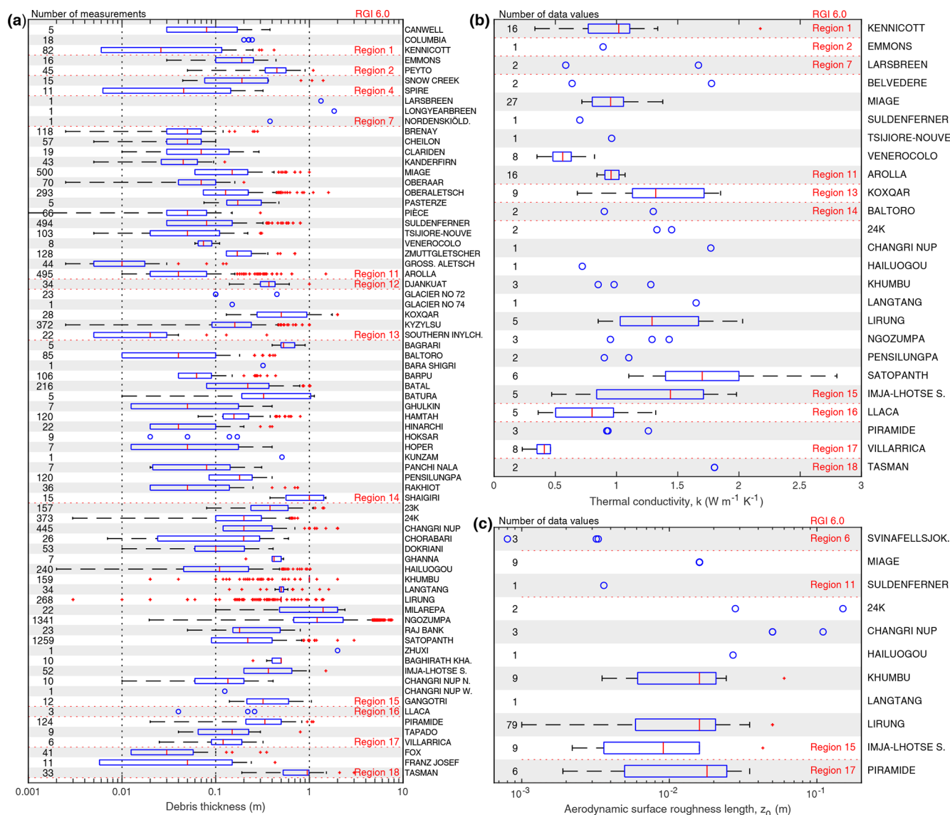
Figure 2. The distribution of debris thickness measurements (a), thermal conductivity (b), and surface roughness length (c) for each glacier in DebDaB. The glaciers are sorted by RGI region (RGI6.0, https://www.glims.org/rgi_user_guide/regions/overview.html , last access: 20 November 2024). The number of measurements or data values are shown on the left. Literature values are not shown. Note the logarithmic x-axis scale for debris thickness and surface roughness length.
