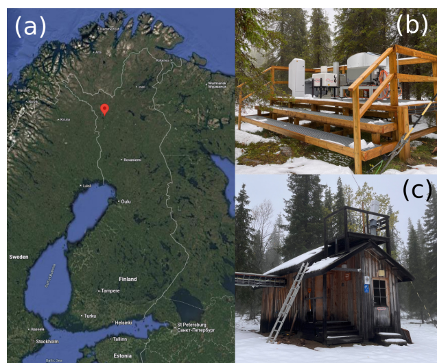
Figure 1. (a) Map of Finland showing the location of the Kenttäröva station (© Google Maps 2024), (b) photograph of the platform with instruments, and (c) photograph of the cabin with a Vaisala CL31 ceilometer on the roof.
