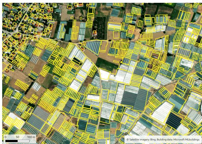
Figure 4. False positive building detection on agricultural lands surrounding Strumica, before filtering of such features.
