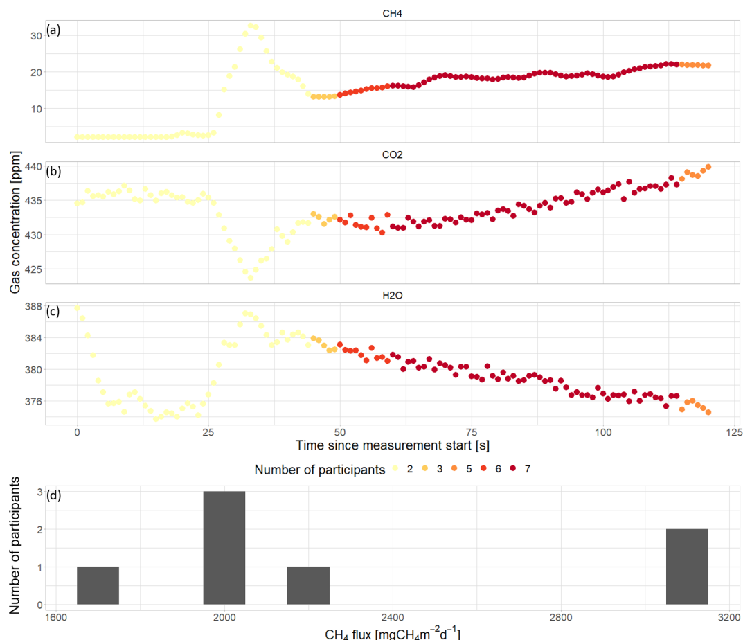
Figure B6. Measurement example (VQC8) of an overall increase in CH 4 concentrations over the time of the chamber closure after a strong jump in CH 4 concentrations. Simultaneous measurements of CH 4 (a), CO 2 (b), and H 2 O (c) concentrations over time during chamber closure, with the colors of the data points indicating how many participants included the respective data point in the time period that they chose for flux calculation. Only the responses by participants who gave start and end times for flux calculation were considered for this figure. Histogram of CH 4 fluxes calculated based on the time period chosen by the participants for flux calculation (d).
