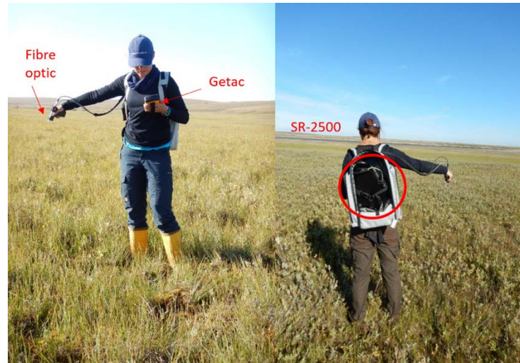
Figure S1: Spectral Evolution SR-2500 field-spectrometer measurement set-up in the Lena Delta, August 2018 (photos: M. Fuchs).
