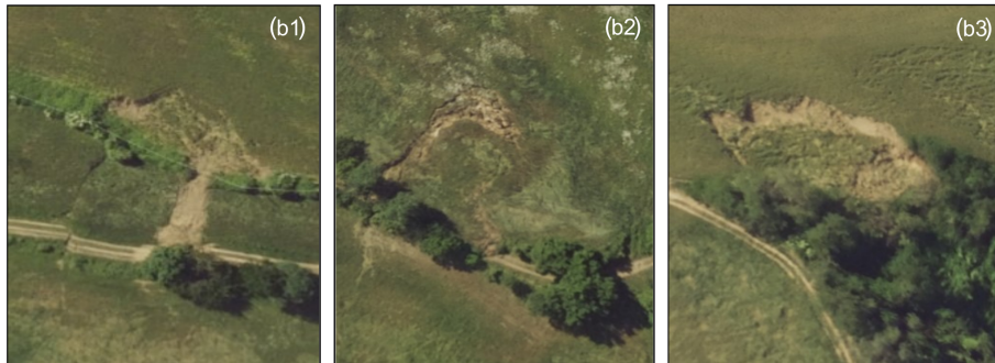
Figure 5. Representative images of the two distinct types of debris slides caused by the May 2023 event.
