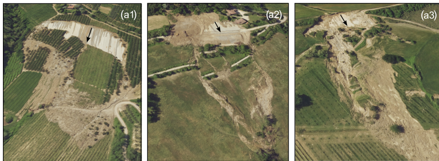
Figure 5. Representative images of the two distinct types of debris slides caused by the May 2023 event.
