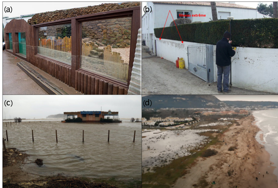
Figure 6. Examples of the level of confidence associated with the flood depth: panels (a) and (b) show a high level of confidence (clear spatial references in the pictures), panel (c) shows a medium level of confidence (some reference in the picture), and panel (d) shows a low level of confidence (no clear reference in the picture). References for the images are as follows: (a) https://www.sealsanctuary.co.uk/pressrel09102014hsls.html (last access: 2 January 2025); (b) http://infoterre.brgm.fr/rapports/RP-58261-FR.pdf (last access: 23 February 2025) (Pedreros et al., 2010; last access: 2 January 2025); (c) https://www.diaridegirona.cat/baix-emporda/2020/01/21/temporal-esborra-les-platges-1-48749485.html (last access: 2 January 2025); (d) https://www.youtube.com/watch?v=oQ5ME3pImmo&list=UUUP8KKIjgWf6JTHg-NNKN9g&ab_channel=CostaBravaVibes (last access: 2 January 2025).
