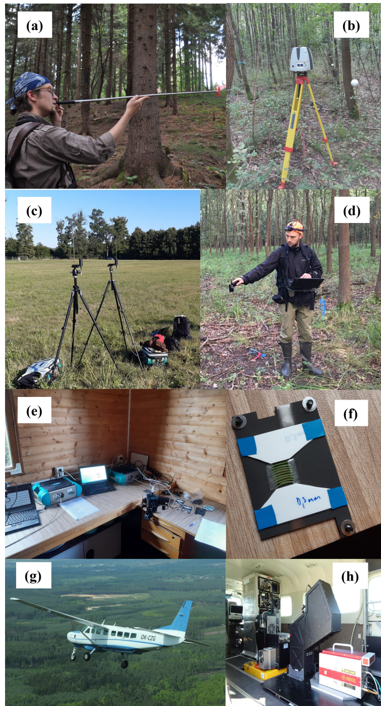
Figure A1. Photographs of different types of measurements conducted during the campaigns. (a) Forest inventory measurements. (b) Terrestrial laser scanning (TLS). (c) Spectral transmittance reference measurements in an open place. (d) Forest floor spectral measurements. (e) Laboratory measurements of the spectral properties of foliage. (f) Needle carriers used in the spectral measurements of foliage. (g) Cessna 208B Grand Caravan aircraft used in the airborne campaigns. (h) View of the sensors inside the Cessna aircraft.
