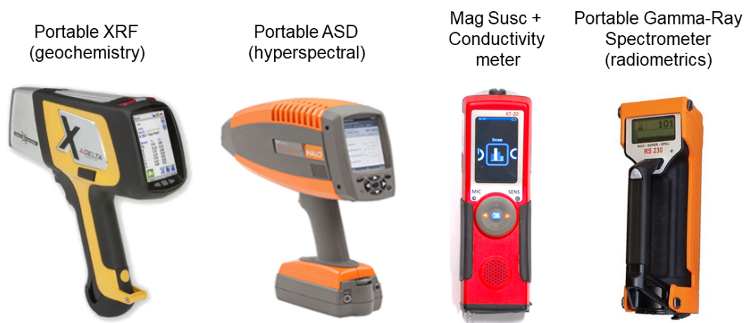
Figure 27. Examples of core-shed tools that can be used for mineral system characterisation and targeting: a portable X-ray fluorescence analyser (pXRF), portable reflectance spectrometer (ASD), magnetic susceptibility and conductivity meter, and gamma-ray spectrometer.
