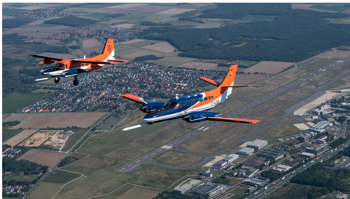
Figure 1. The research aircraft Dornier 128 D-IBUF (left) and Cessna F406 D-ILAB (right) with striking colours for good visibility and the characteristic nose boom for meteorological measurements flying above their home base, the Braunschweig airport. Photo by Florian Szczepanek, https://www.aviation-media.com/ (last access: 15 October 2024).
