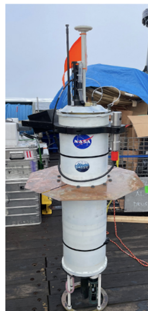
Figure 33. The under-ice float (UIF) on the deck of R/V Woldstad before deployment. The float is about 2 m tall from the deck to the top of the antennas. Note CTDs at top and bottom of the float, the upward-looking camera mounted near the top of the float body on the left, and an ice-profiling sonar attached to the right-hand side. Photo credit: Jim Thomson.
