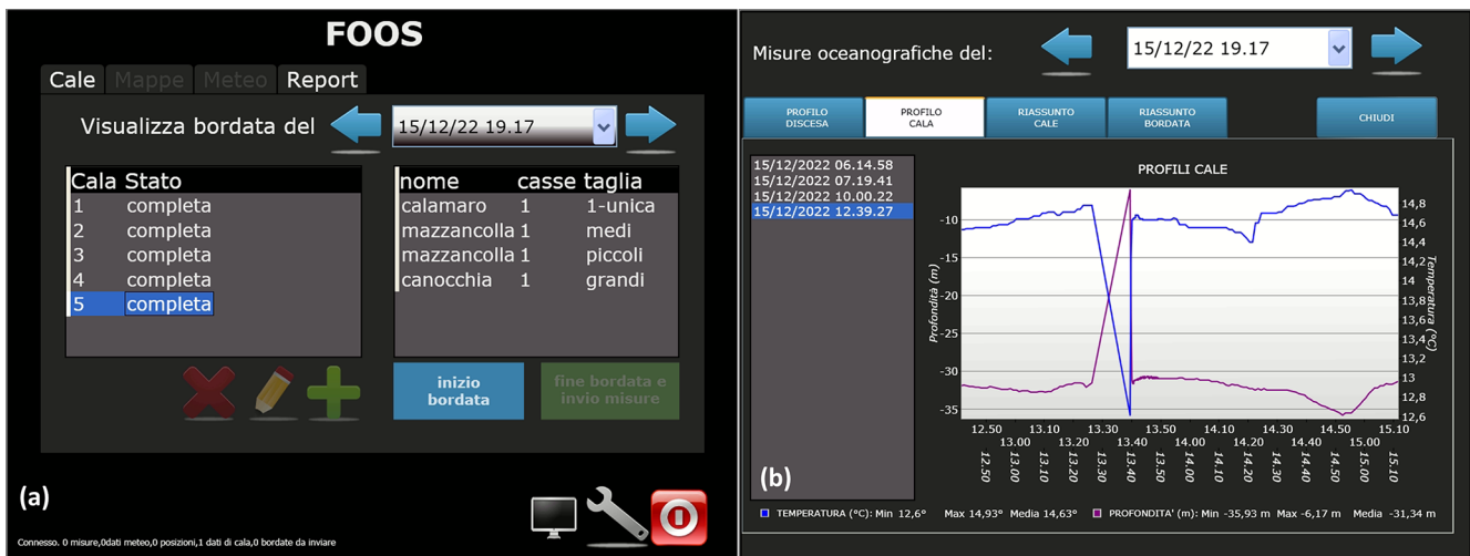
Figure 4. AdriFOOS GUI used on board by fishers: screenshot examples from the catch module (a) allowing the user to enter the start and end of the trip (in Italian inizio and/or fine bordata ) and caught species quantity ( casse ) and size ( taglia ) by haul ( cala ). The oceanographic real-time data visualization module (b) showing fished depth (purple line) and relative temperature (blue line) by haul.
