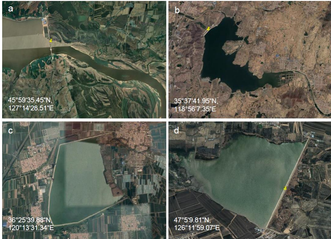
Fig. S1. Types of dams/reservoirs in this study. (a-b) On-stream dam/reservoir constructed on a river/stream regardless of impoundment; (c-d) Off-stream dam/reservoir formed by partial or complete embankment around an off-stream lake. The high-resolution images in this figure were from the Google Earth Pro (© Google Earth Pro 2019).
